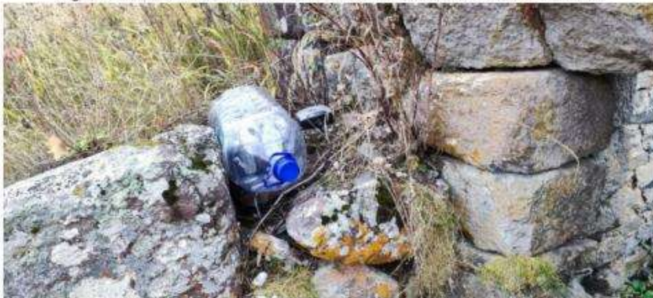
Figure 8.1: Vibration monitor SWARM was installed outside on the wall of the Tower
